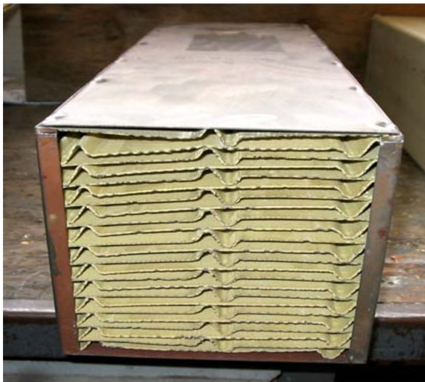
Figure 3-2 Plate Catalyst Bench Scale Test Module 6
