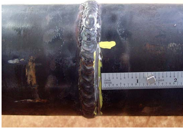
Figure 3-6 Flaw #4, 30% around the Circumference and 30% Through Wall
