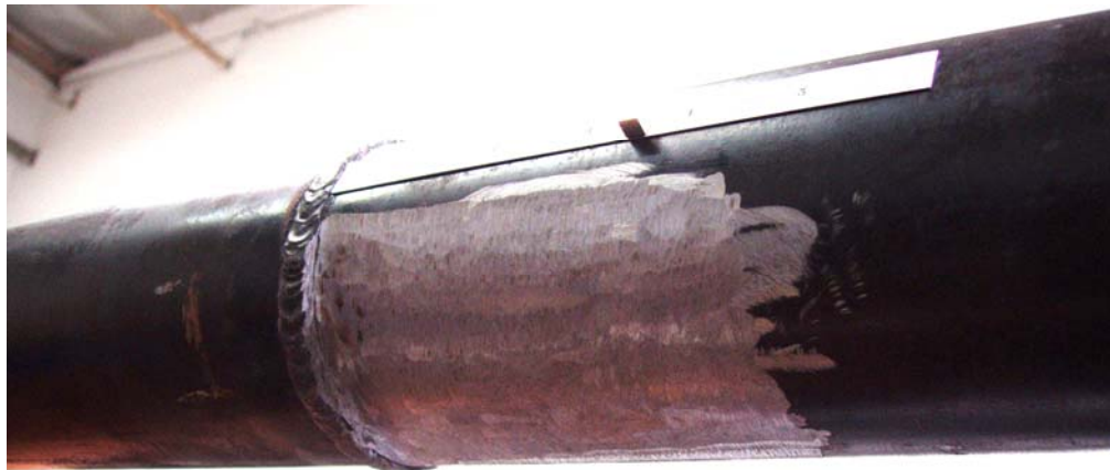
Figure 3-3 Flaw #2 Simulated Axial Wall Loss Associated with a Girth Weld
