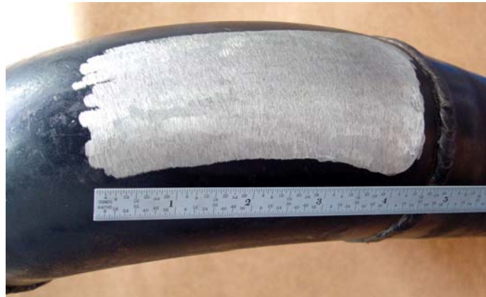
Figure 3-4 Flaw #3, Simulated Wall Loss in an Elbow
