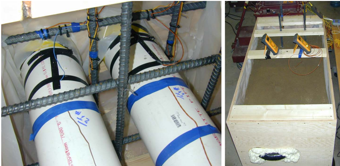
Figure 5-2 Test Setup: Steel Reinforcing Rods and Temperature Measurements
