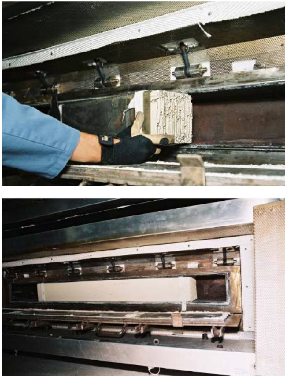
Figure 2-2 Photographs of Laboratory Test Reactor with Catalyst Sample
