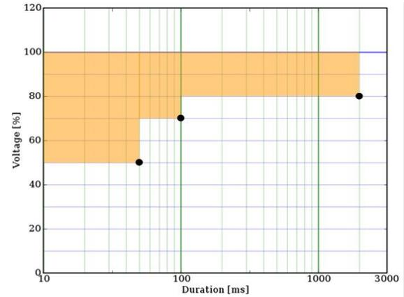
**Type I and II voltage sag test points:**
