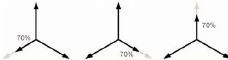
Figure 2-4 Phase-to-Neutral Voltage Sags
