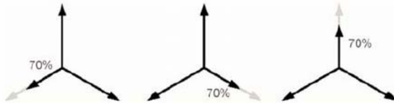
Figure 2-4 Phase-to-Neutral Voltage Sags
