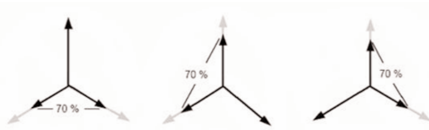
Figure 2-6 Two-Phase-to-Neutral Voltage Sag Type
