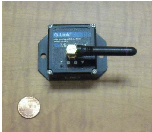
Figure 5-11 Vibration sensor and wireless communication unit
