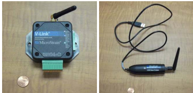
Figure 5-9 Wireless communication unit (left) and receiver to computer (right)
