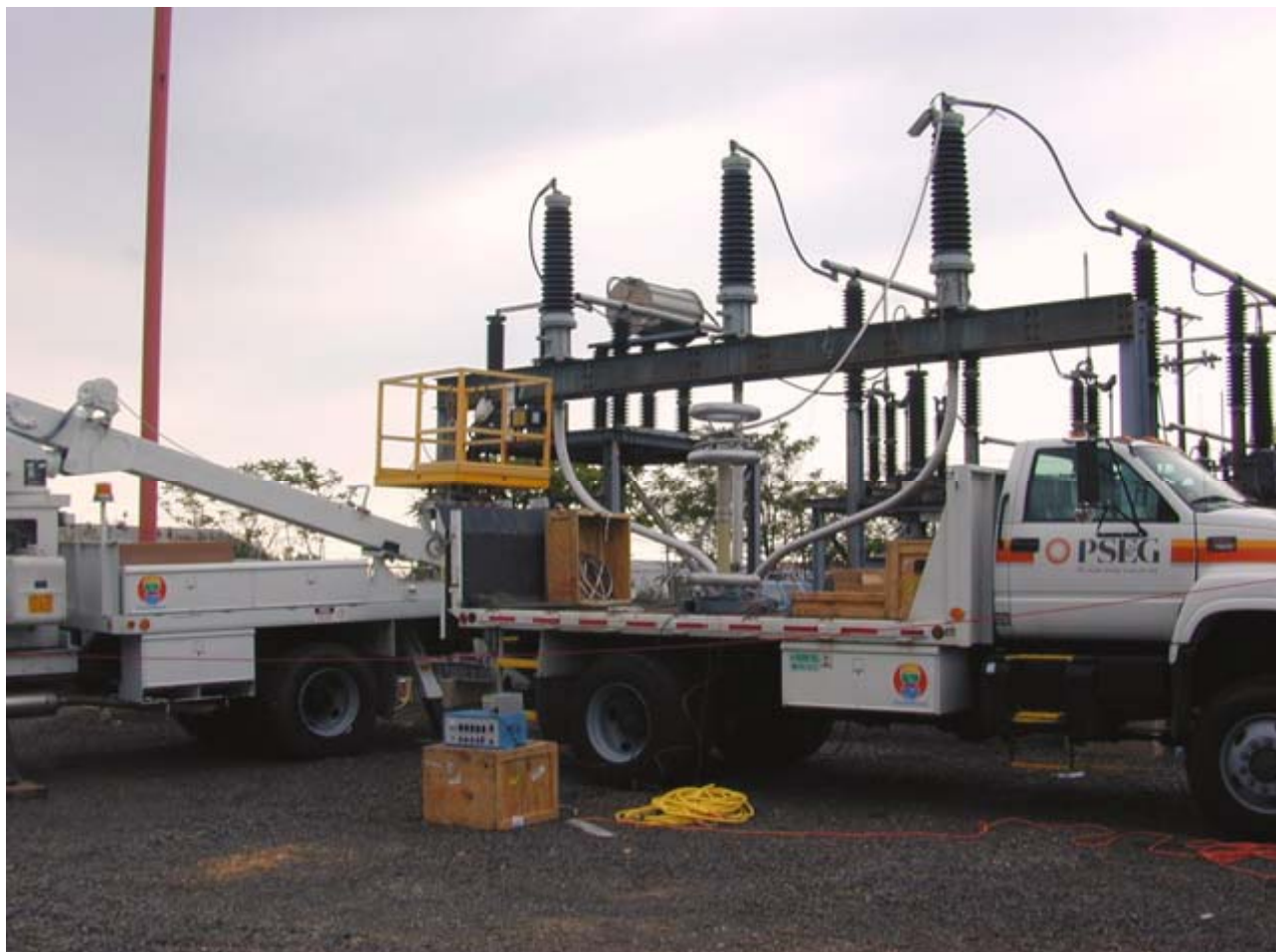
Figure A-8 Dissipation Factor Measurements at the PSE&G North Avenue Substation
