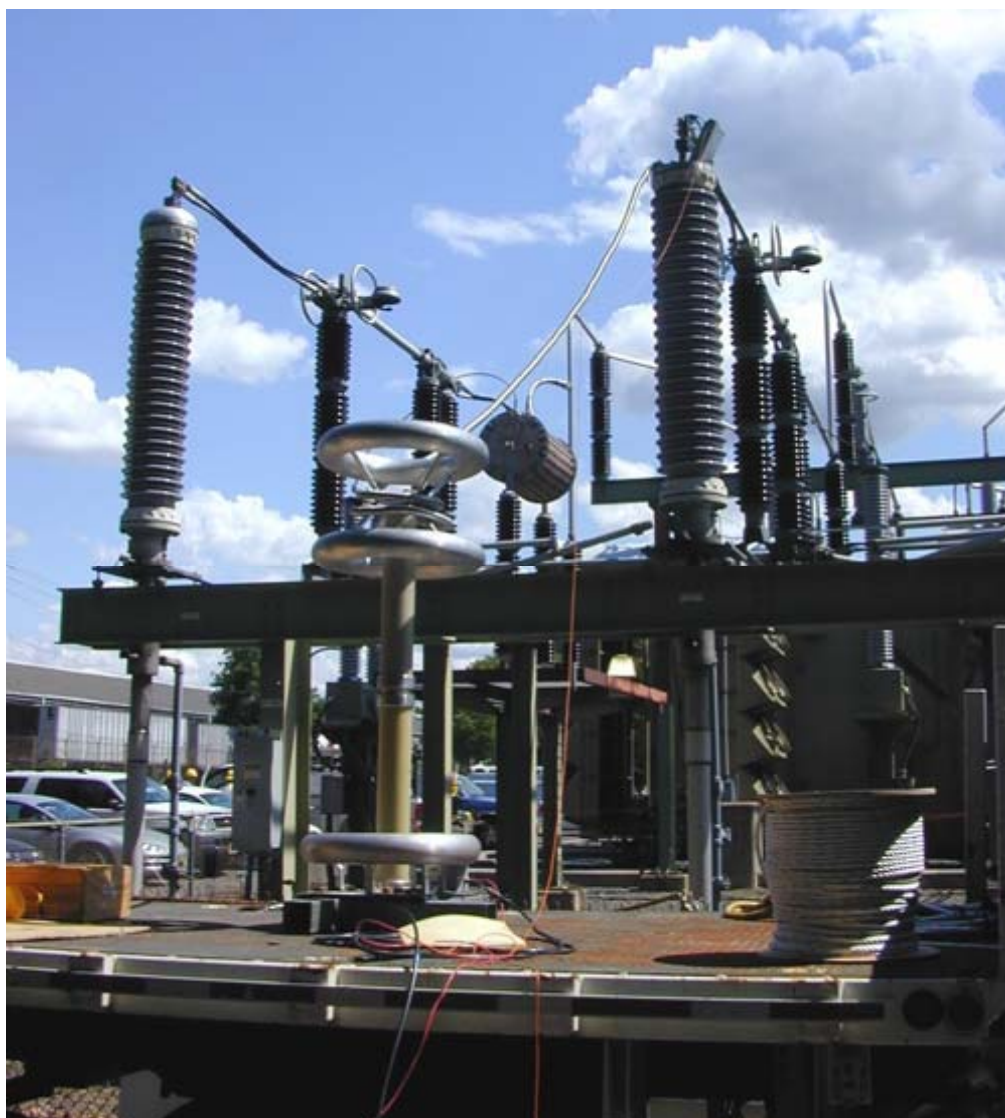
Figure A-7 Dissipation Factor Measurements at the PSE&G Fairlawn Switching Station
