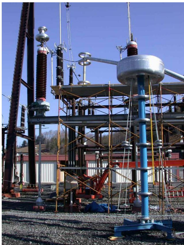
Figure A-9 Blenheim–Gilboa Cable #3 dissipation factor measurements
