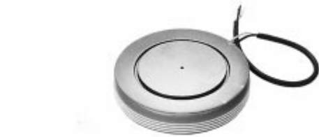
Figure 2-2 Photograph of the World's Highest Voltage Semiconductor Device – Mitsubishi FT1500AU-240 6,7
