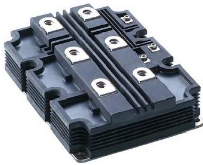
Figure 2-6 Photograph of ABB 5SNA0600G650100 High-Voltage IGBT
