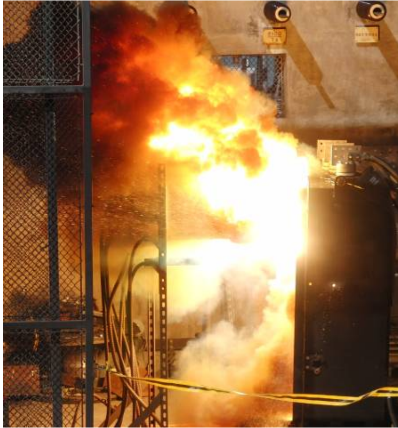
Figure 1-6 Example 480-V Network Protector Event
