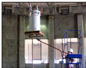
Figure 5 Laboratory measurement of the vertical magnetic field profile near a pole-mounted transformer
