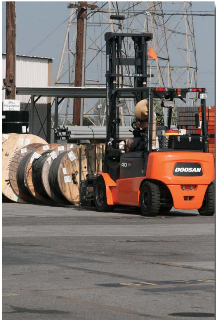
Doosan Electric Outdoor Forklift, 8,000 lb. Capacity
