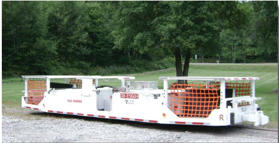
A. L. Lee Corporation 9RR-B Battery Powered Rail Runner
