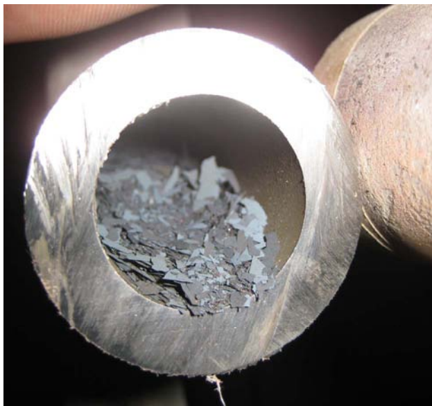
Figure 1-2a Magnetite flakes in lower tube bend
