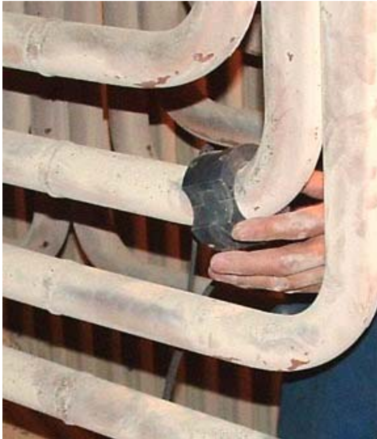
Figure 1-3 Russell NDE Systems electromagnetic inspection probe on secondary super heater outlet tube
