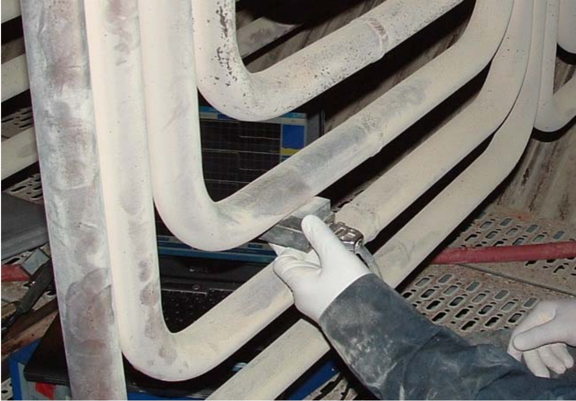
Figure 1-8 TestTex LFET inspection probe on a secondary super heater outlet tube
