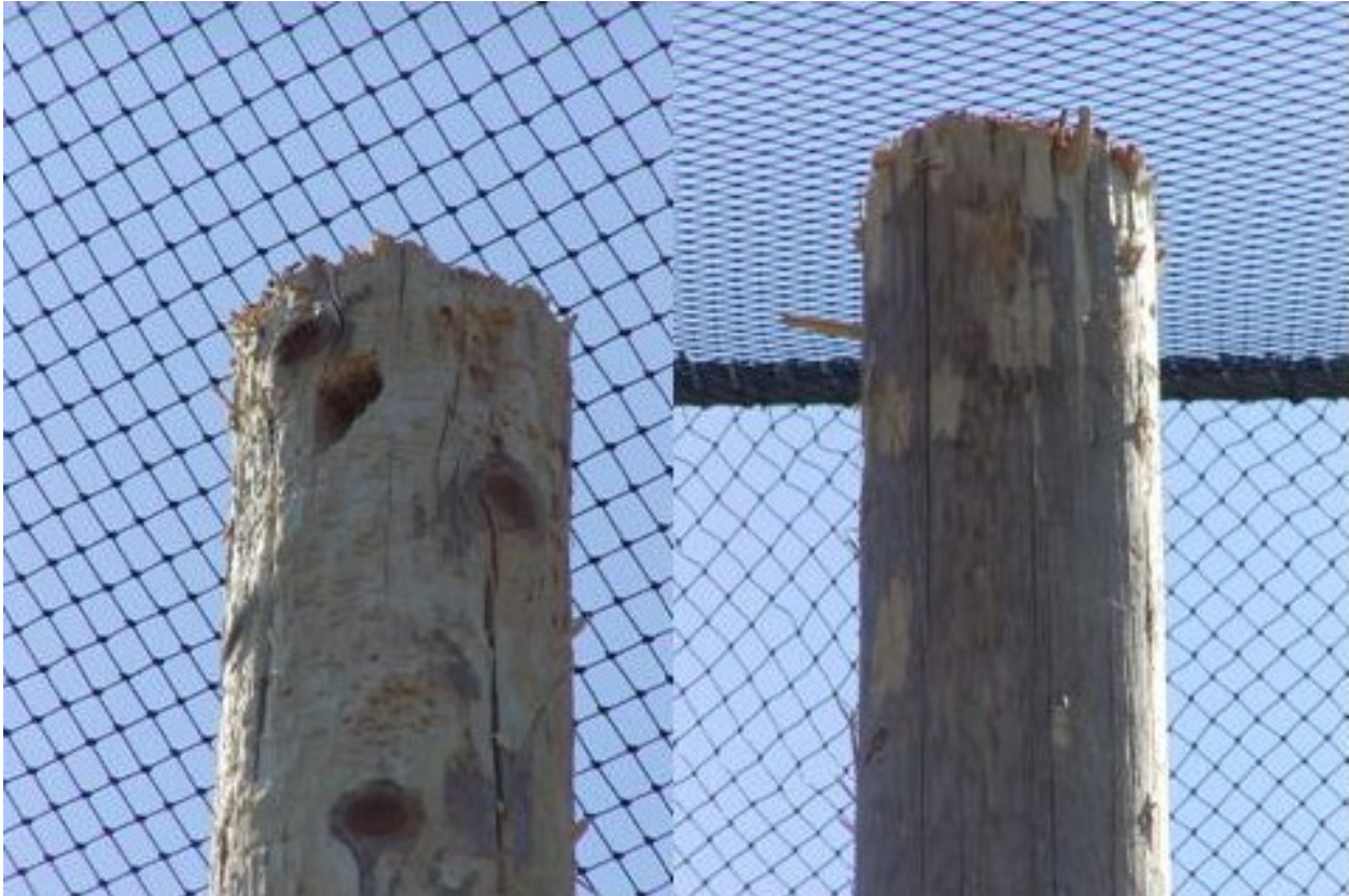
Figure 4-1 Photo of Bird 5 Test Poles (Sonic Dissuader Pole at Left, Control Pole at Right) from Testing Conducted at NWRC from 14 August through 05 October 2007
