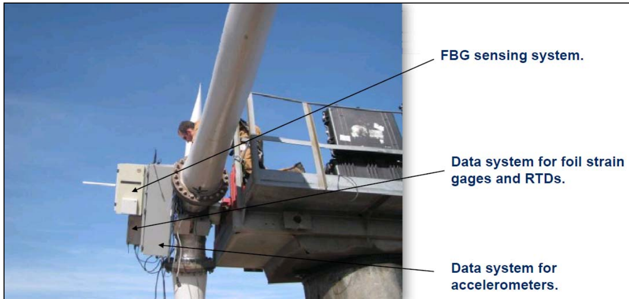
Figure 3-2 Test Turbine for the Sandia Sensor Blade Project in Bushland, Texas [14]
