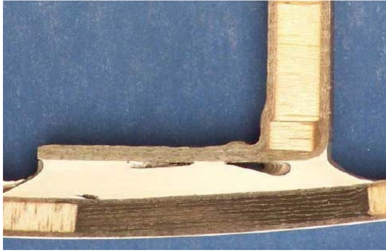
Figure 2-6 Voids in an Adhesive Bond between a Spar Cap and the Flange of a Shear Web [20]
