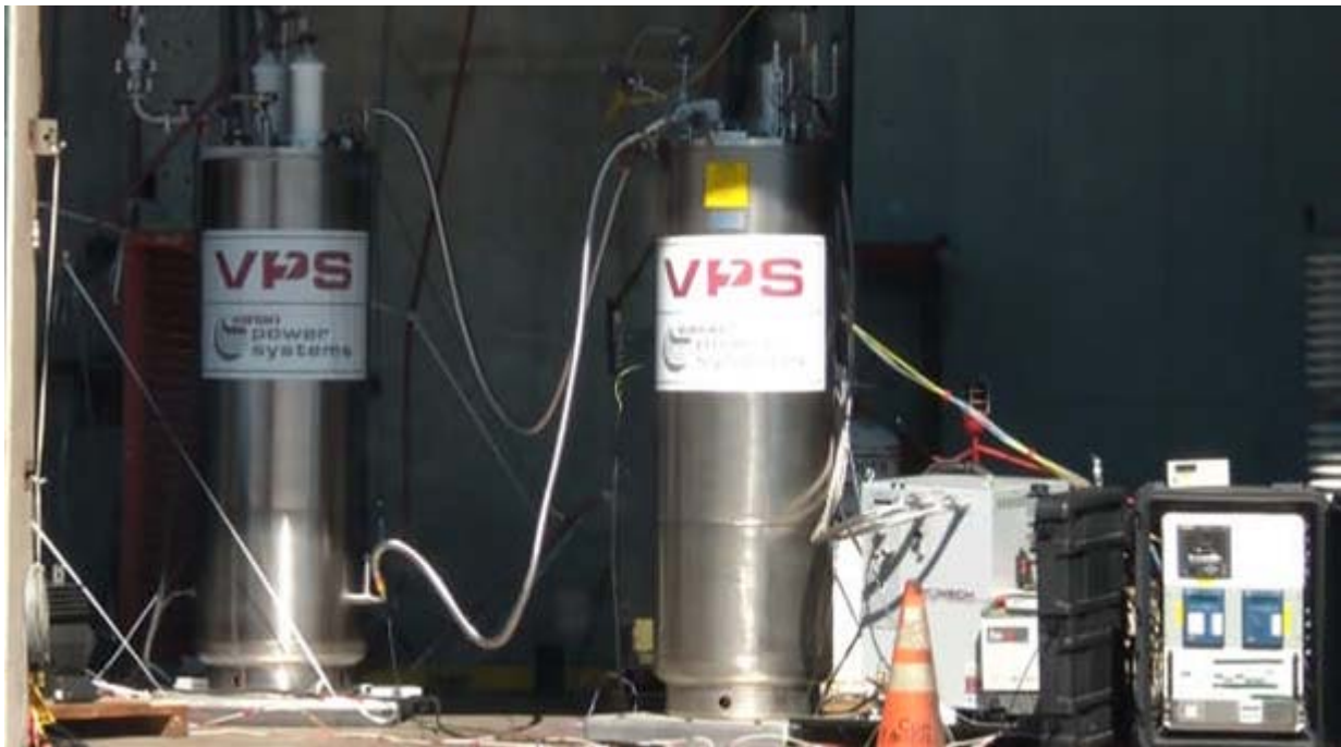
Figure 3-2 Varian superconducting fault current limiter under fault testing at KEMA, Chalfont, PA Used with permission from Varian Power Systems
