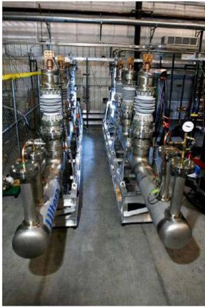
Figure 2-8 25 m prototype test at the ORNL: terminations (left), cable loop (right) Source: High Temperature Superconducting Cable, 2009 DOE Peer Review, August 4–6, 2009. Alexandria, VA
