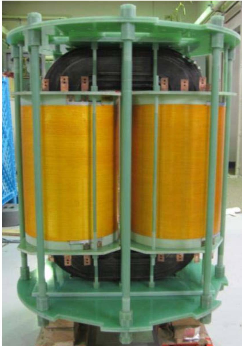
Figure 3-8 One phase of Nagoya 2 MVA superconducting fault current limiter transformer Courtesy of the Electric Power Research Institute
