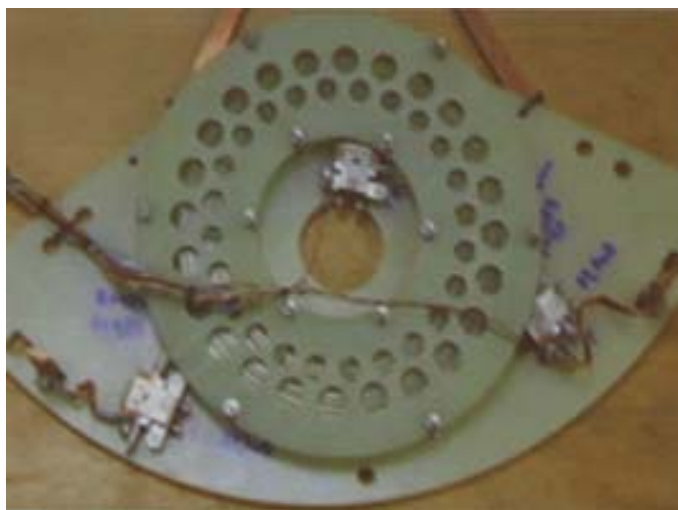
Figure 2-11 The Nexans YBCO tape element for the Boxburg Courtesy of Electric Power Research Institute
