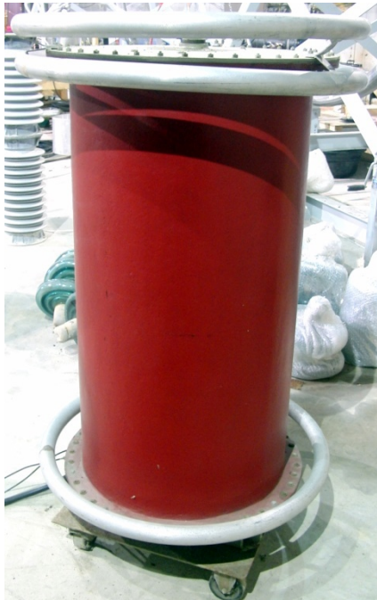
Figure B-6 Hipotronics HVAC Transformer.
