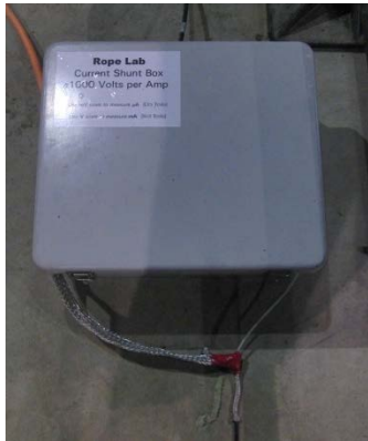
Figure B-2 Leakage Current Shunt Box.
