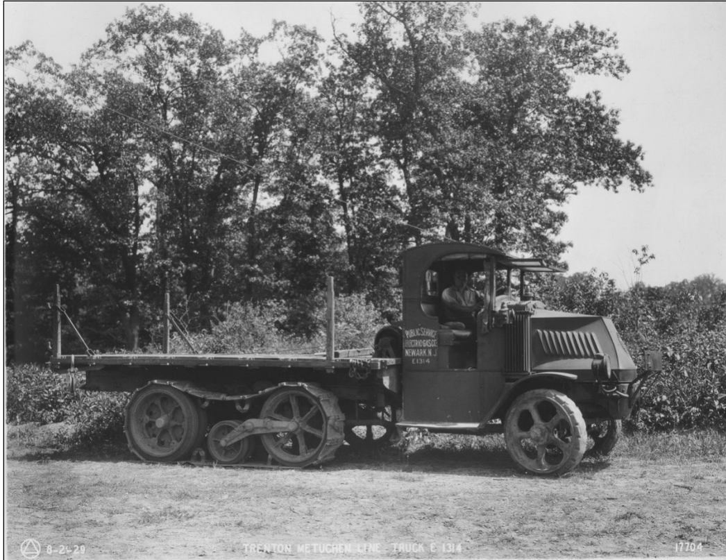
Figure 1-1 Live Line Maintenance Truck, circa 1920s.
