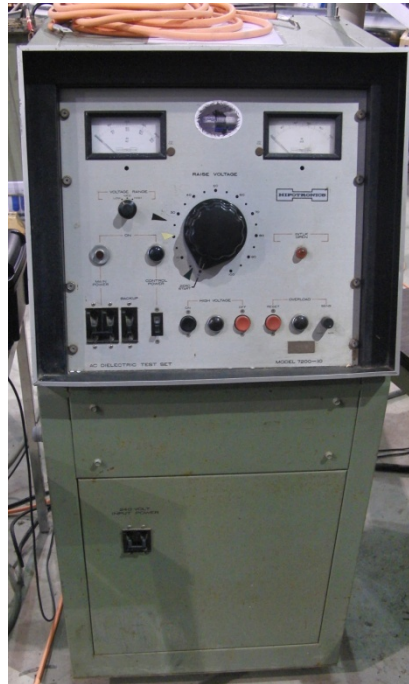
Figure B-7 Hipotronics HVAC Control Box.
