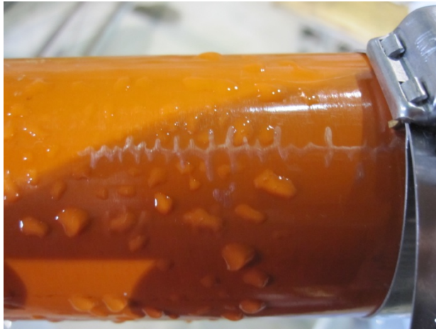
Figure 5-12 Local De-Lamination after One Wet Energized Test.
