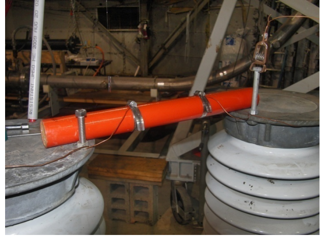
Figure 5-2 Close-up View of a Sample of a LW Tool under Test
