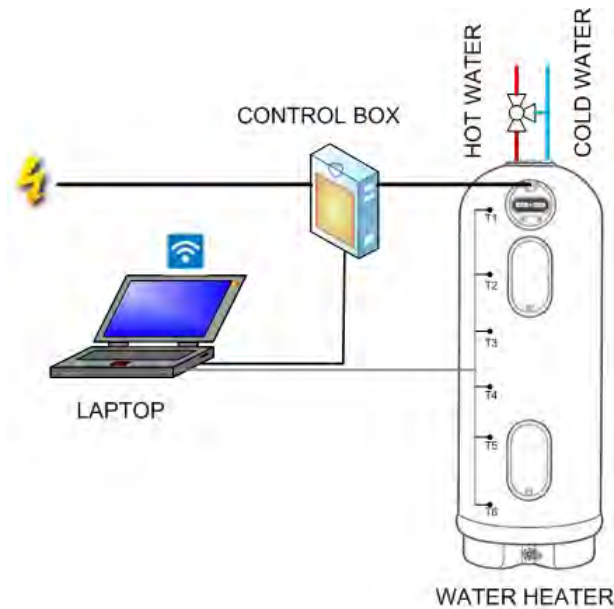
Figure 5-2 Schematic of Steffes Grid Interactive Water Heater
