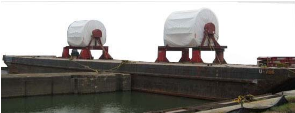
Figure 2-2 Turbine Rotors on Barge for Shipment
