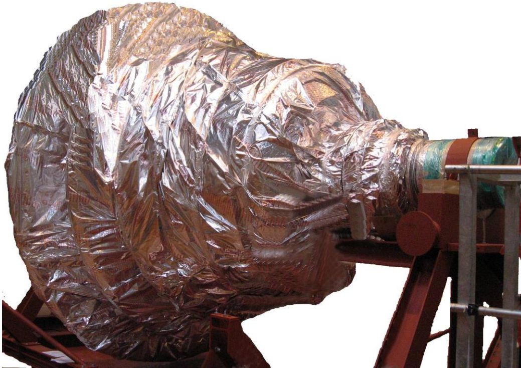
Figure 3-3 Turbine Rotor Stored in Shrink Wrap
