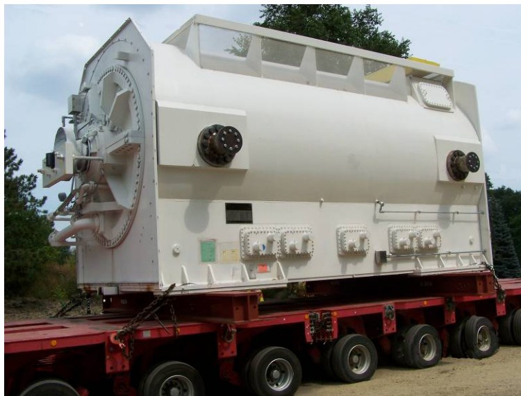
Figure 2-7 Stator Shipping by Truck Example (Picture courtesy of XCEL Energy)
