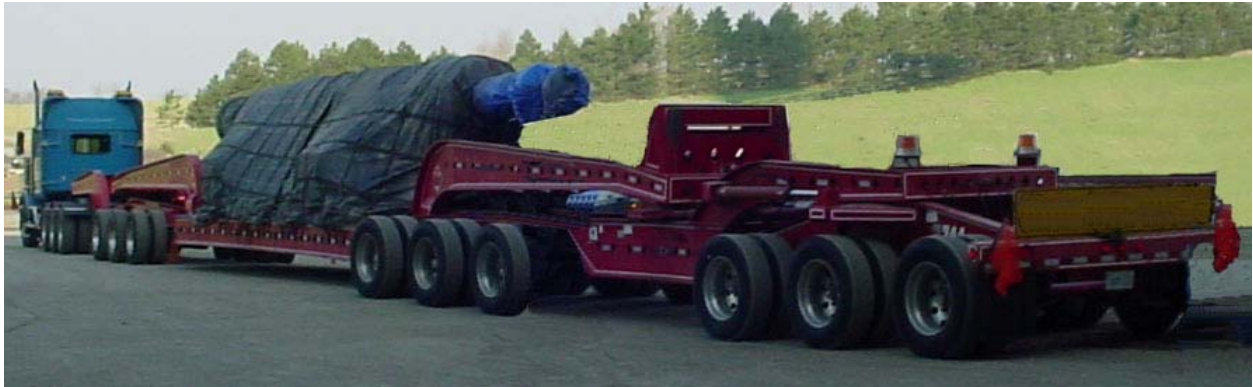
Figure 2-4 Generator Rotor Truck Shipping Example (Picture courtesy of Alliant Energy)
