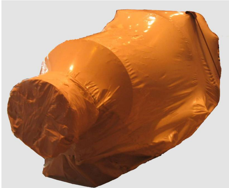
Figure 2-9 Exciter Prepared for Shipment and Storage Example (Picture courtesy of Dominion)
