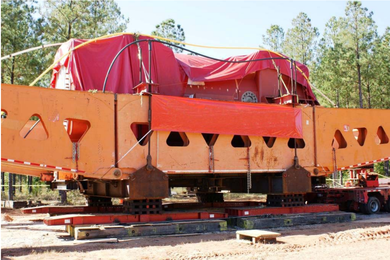
Figure 2-6 Stator on Heavy Haul Trailer (Picture from P3 files)
