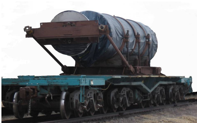
Figure 2-5 Generator Rotor Rail Car Shipping Example (Picture courtesy of Exelon Corporation)
