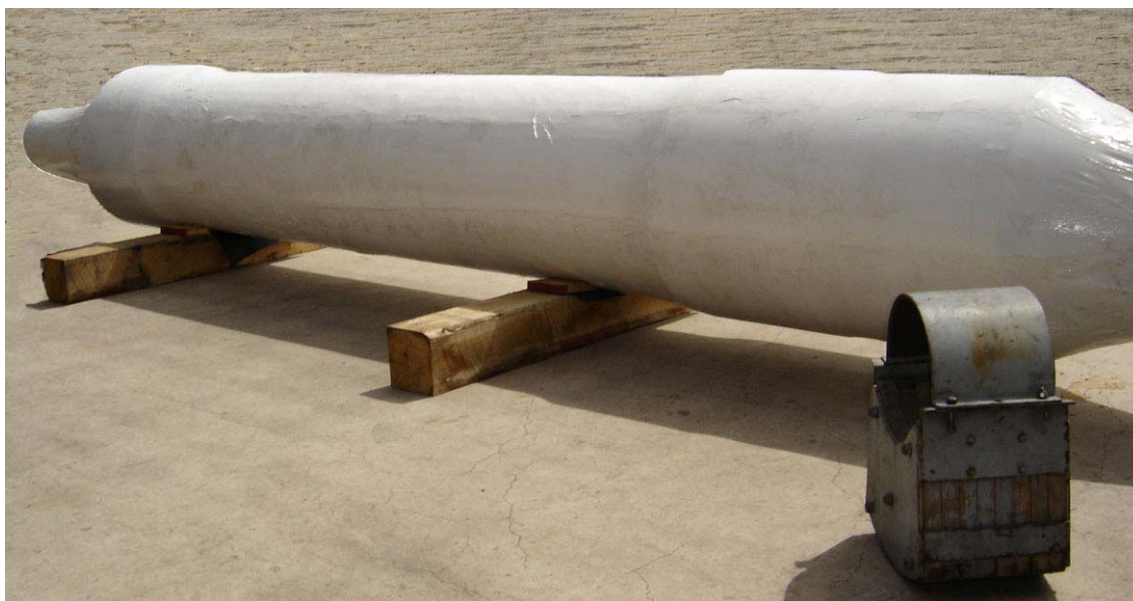
Figure 3-5 Generator Rotor Shrink Wrap Storage (Picture courtesy of NV Energy)
