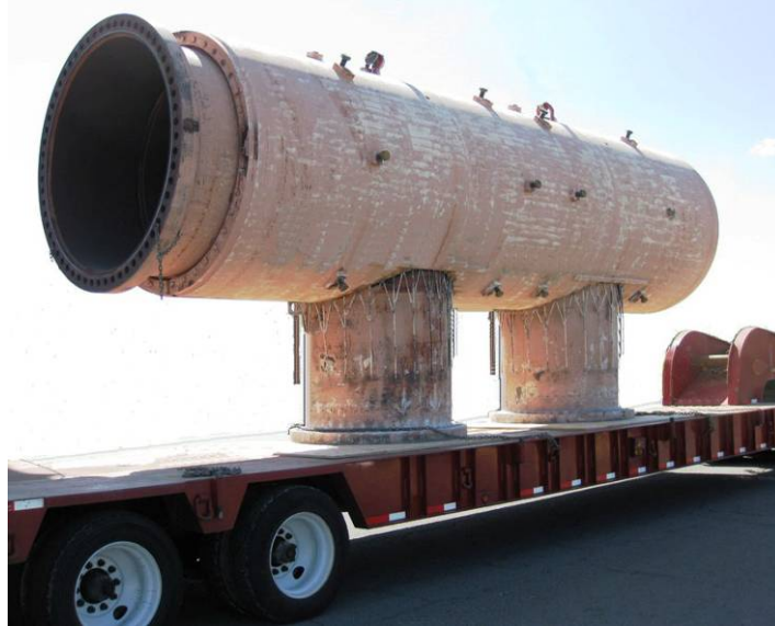
Figure 2-8 Crossover Pipe Shipping Example (Picture courtesy of Entergy Corporation)
