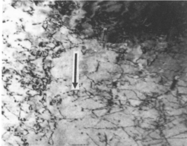
Figure 2-1 Evidence of dislocation loop in polycrystalline iron. [8]
