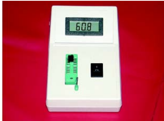
Figure 3-6 Example of a tool used to measure the ratio between output current and input current.
