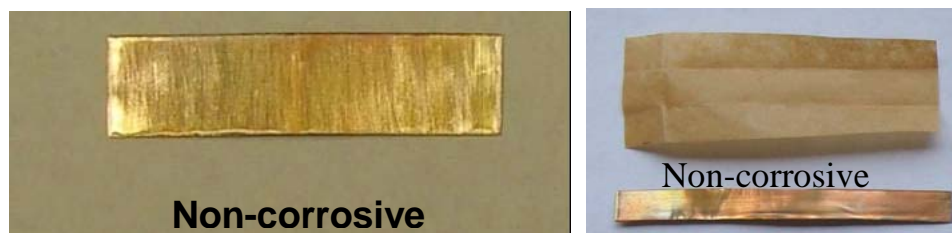
Figure 2-7 Test Results from the ASTM 1275B (left) and CCD-ABB Corrosive Sulfur Tests (Right) of Oil #2 After Treatment.
