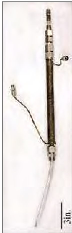
Figure 2-1 Schematic and Photograph of External Pressure Balanced Ag/AgCl Reference Electrode.
