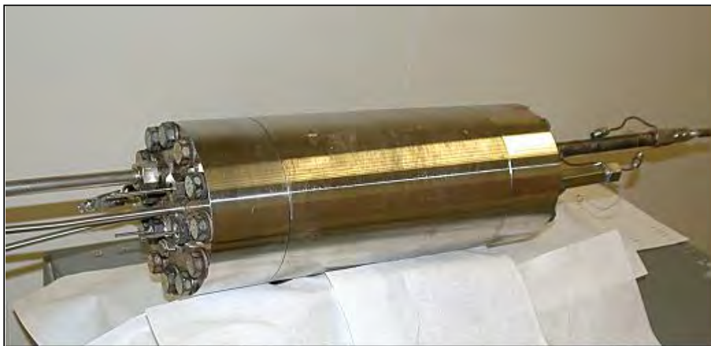
Figure 2-6 Autoclave Immediately After Sealing with Test Solution
