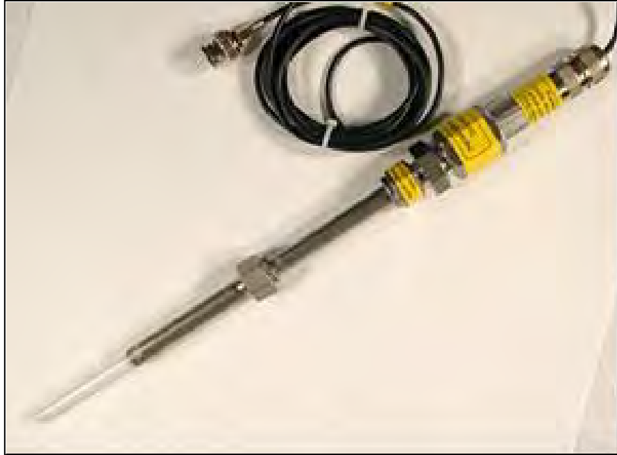
Figure 2-2 Photograph of yttria-stabilized Zirconia pH Sensor
