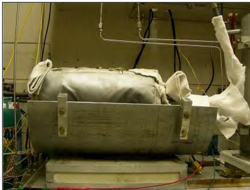
Figure 2-7 Autoclave Enclosed in Thermal Blanket and Seated in Bottom Section of Clam Shell Blast Shield
