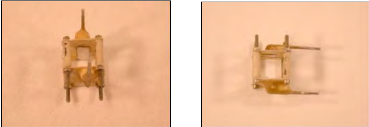
Figure 2-3 Views of Conductivity Cell Used in High Temperature Solutions
