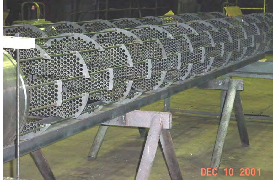
Figure 4-14 Tube bundle cage structure prior to tube insertion
