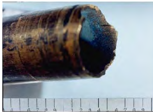
Figure 4-4 Sheared tube due to stress corrosion cracking
