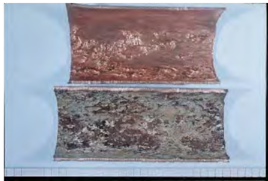
Figure 4-6 Copper alloy tube with ID pitting and erosion
