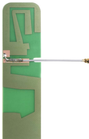
Figure 5-1 This quad-band antenna supports 4 different frequency bands listed in Table 5-1
