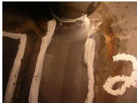
Figure 10-6 Identified areas that might require additional testing
