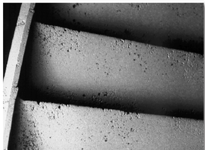
Improved understanding and quantitative characterization of corrosion fatigue damage underlies a new remaining life assessment approach for steam turbine blades in fossil and nuclear power plants.
