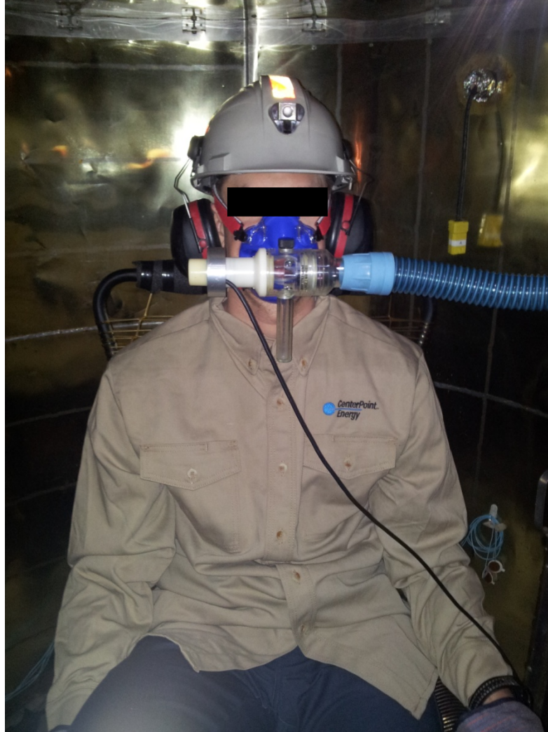
Figure A-1 Subject sitting in calorimeter
