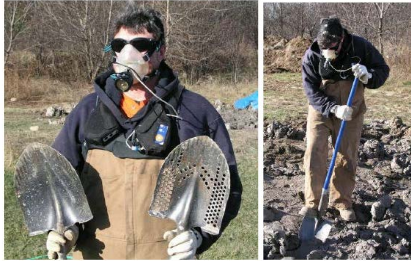
Figure 6-1 An example of the use of a portable metabolic system to measure energy expenditure in the field.
