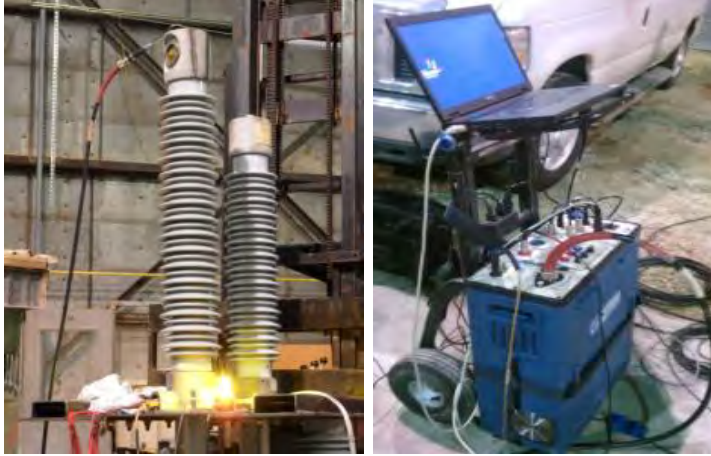
Figure 6–5 Power Factor Testing Set-Up at EPRI's Lenox Facility
