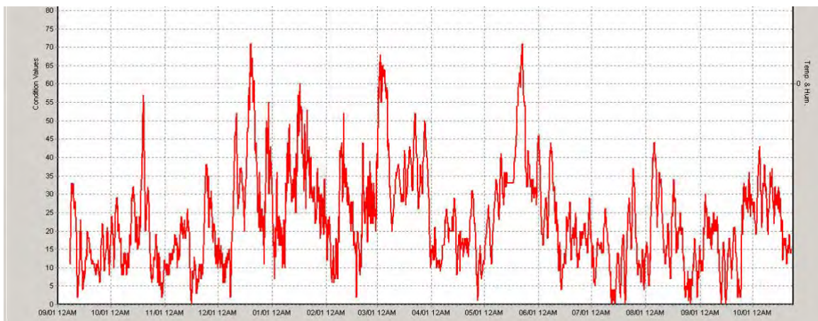
Figure 11–21 Condition Value Trend for the H2 Bushing
