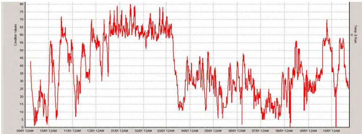
Figure 11–24 Condition Value Trend for the X2 Bushing
