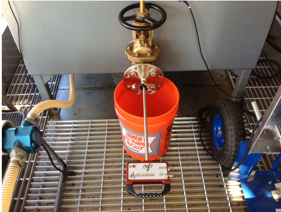
Figure 7-2 Drain Valve UHF Probe Manufactured by NDB Technologies (Supplied as Part of Their AE-150 System)
