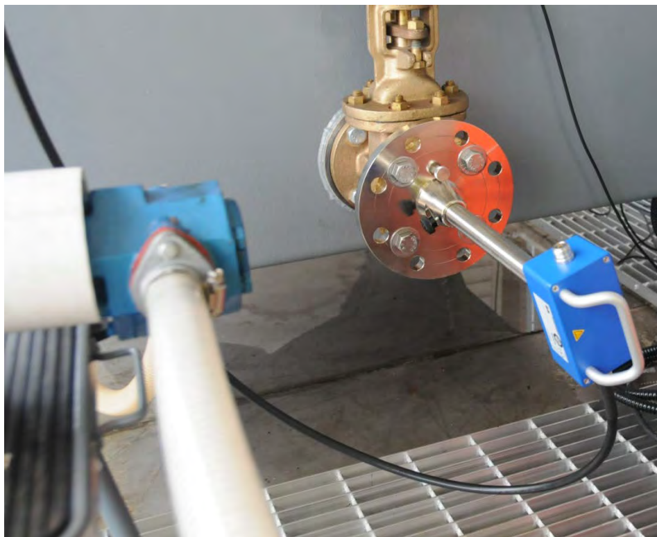
Figure 7-3 Omicron Drain Valve UHF Probe UVS610 Supplied as an Option to the MPD600 Measurement System
