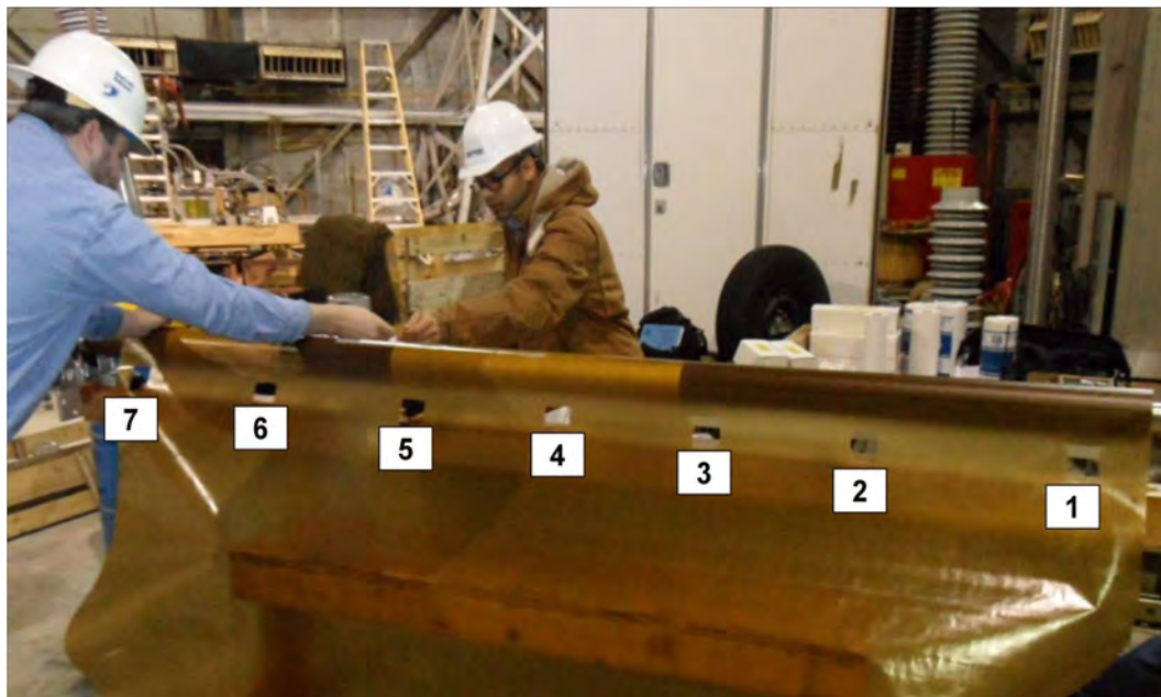
Figure 6–10 Samples were Obtained Axially along the Length of the Core at Regular Intervals
