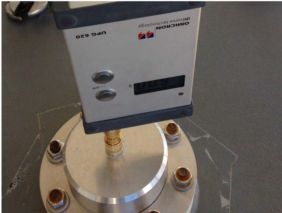
Figure 7–1 UHF Calibrator Injecting Signals into the UHF Sensor Mounted to the Lid of the Test Transformer (Sensor Designated U04)
