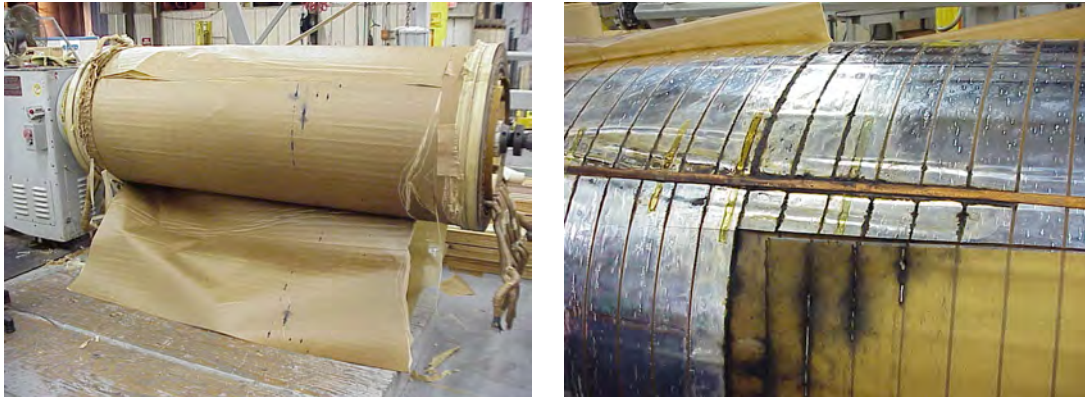
Figure 11-2 Insulation Damage Found by Unwinding Coil Assembly
