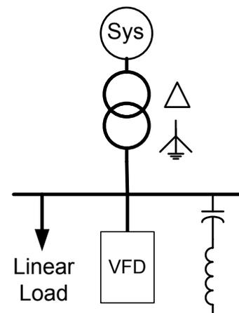
**Harmonic filters designed for radial power systems should be designed to accommodate loadings associated with background harmonic voltage levels that are compliant with IEEE 519 standards.**
