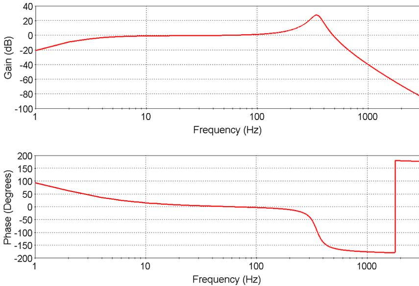
The graphs show the gain is unity (0 dB) and the phase angle is zero at nominal frequency. However, at harmonic and interharmonic frequencies, the per-unit output of the CCVT varies significantly from its input. The table below shows the resulting gain and percent measurement error for several common harmonics.
