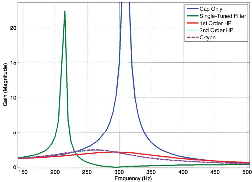
An important feature of this figure is to show the relative change of various frequency components; however, to truly evaluate the effects of the shunt device, either measured or estimated background harmonic voltage data must be available. The table below shows the background harmonic voltage levels, resulting harmonic voltage (Vh) levels, and percentage of total harmonic voltage distortion (%Vthd), once a particular shunt compensator is connected to the 115kV bus.
