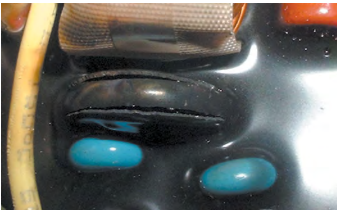
This potted MOV failed as a result of a TOV incident upon the AC line input.
