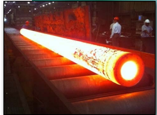
Hot extrusion of an Inconel® Alloy 740H (ASME Code Case 2702) Pipe at Wyman-Gordon Pipe and Fittings, Houston, Texas. The 15,000-pound ingot was cast by Special Metals Corporation, Huntington, West Virginia. The alloy is the prime candidate for advanced ultrasupercritical steam boilers. (Photo courtesy of Wyman-Gordon Pipe and Fittings)
