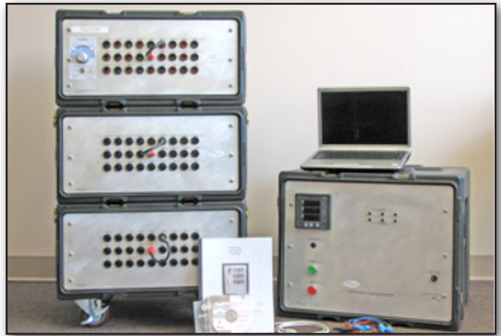
Modular, Tri-mode Porto-Sag for Performing Line-to-Line and Line-to-Neutral Sag Tests
