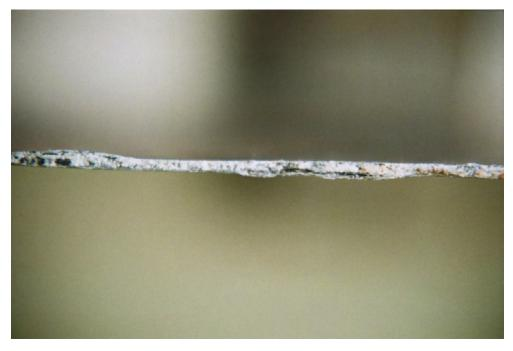
Figure 3-7 Oxidized Edge of BORAL® [1]
