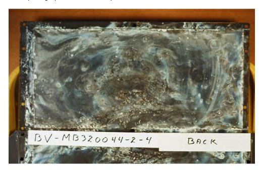
Figure 3-4 Macrophotograph of  ${\it BORAL}^{\it @}$  Coupon with Localized Corrosion –  ${\it Back Side}$  [1]
