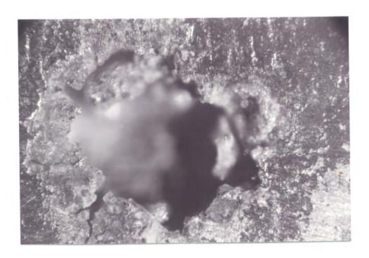
Figure 3-6 Through-Cladding Corrosion Pit [1]
