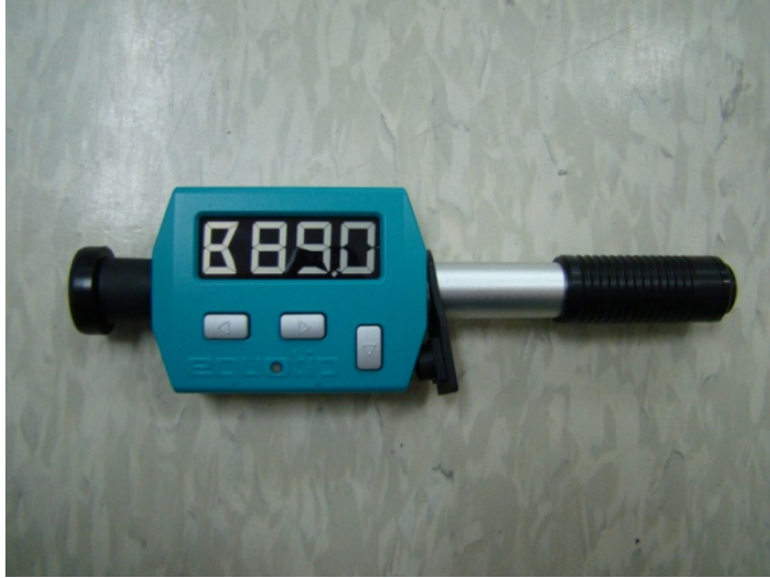
Figure 2-2 Equotip Portable Hardness Tester Used for Brinell Hardness Testing
