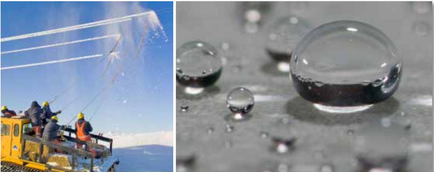
Figure 5 – Hydrophobic coatings help components shed precipitation, mitigating water damage and facilitating ice removal.
