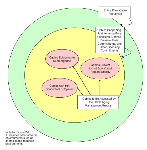
Figure 2-1 Medium-voltage cable circuit scoping process
