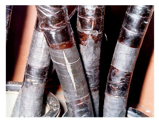
Figure 3-1 Jacket cracking can be seen on these power cables in a motor terminal box that are thermally aged. Thermal aging combined with manual manipulation during maintenance ultimately led to an in-service failure
