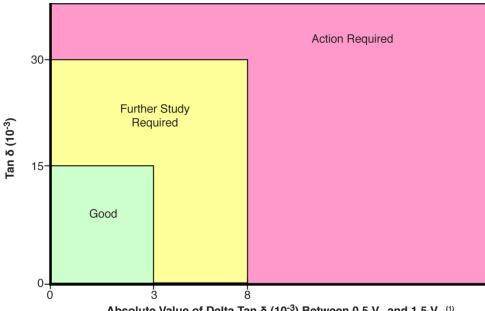
Absolute Value of Delta Tan  $\delta$  (10  $^{\!\!\!-3}\!\!\!)$  Between 0.5  $V_0$  and 1.5  $V_0$   $^{\!\!\!\!(1)}$
