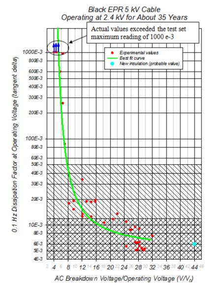
Figure 5-5 Graph showing the inverse relationship of ac breakdown to 0.1-Hz tan  $\delta$  magnitudes for service-aged cables in wet environments. The blue data point is the expected ac breakdown strength of a new cable
