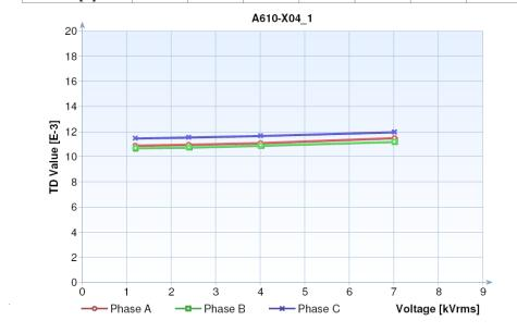
Figure 5-2 Typical "good" tan  $\delta$  result for a shielded cable with pink ethylene propylene rubber insulation
