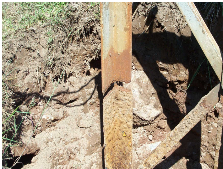
Figure 2-8 Sulfate-reducing bacteria colonizing a tower leg with tubercles
