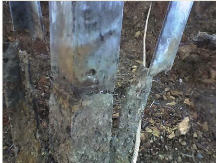
Figure 2-11 Direct current stray current corrosion (long-line effects)
