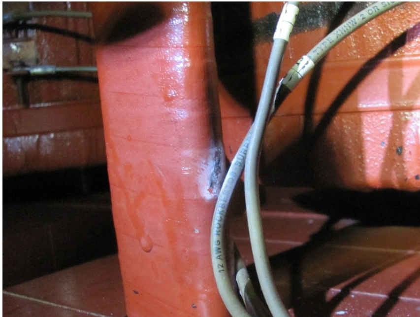
Figure 1-12 Partial arc indication on current transformer cable and phase bar of a 13.8-kV motor
