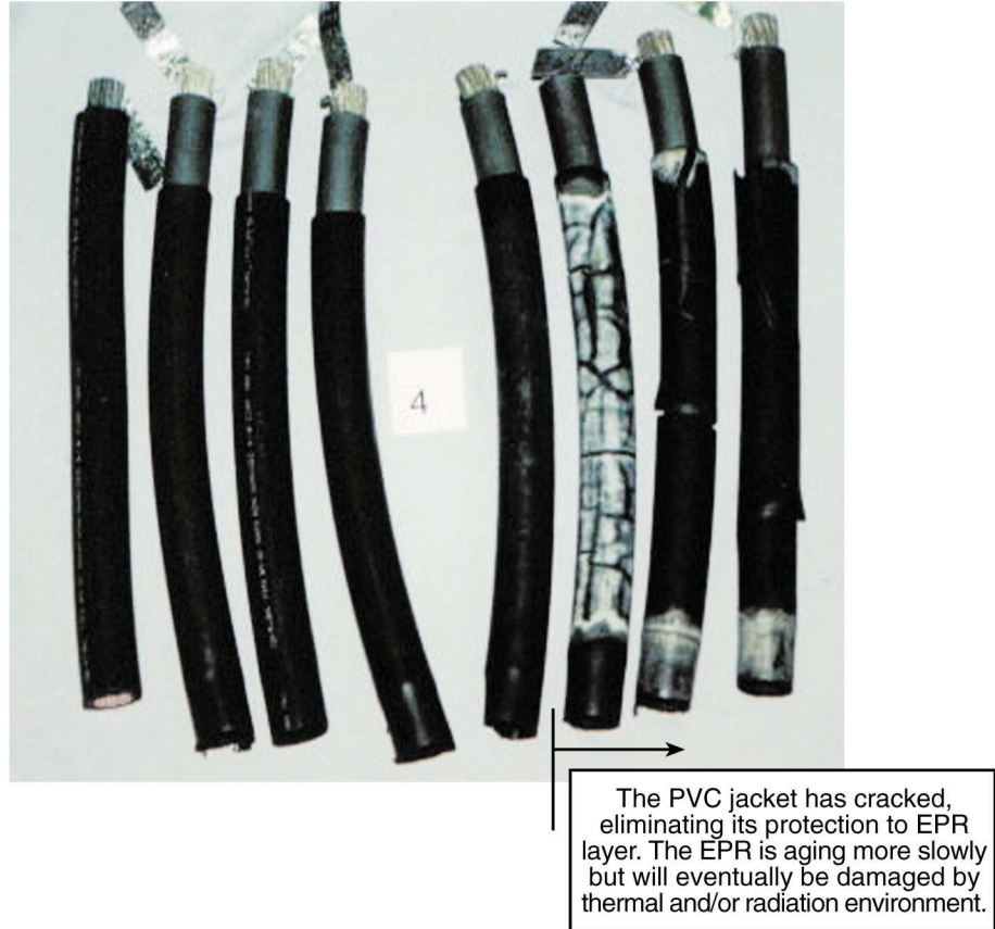
Figure 6-2 Progressive Aging of PVC Jacket and EPR Insulation When Exposed to the Same Environments
