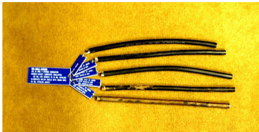
Figure 6-3 Aged Hypalon Jackets on Cables with Bonded Jacket EPR/Hypalon-Insulated Conductors
