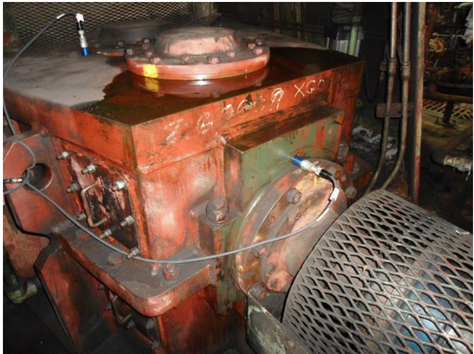
Figure 2-3 Pulverizer gearbox accelerometers
