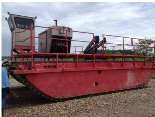
Figure 5-3 Overwater rig for CPT deployment (courtesy AEP)
