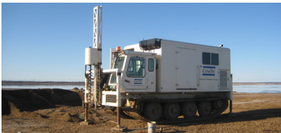
Figure 5-2 Tracked CPT rig (photo courtesy of Conetec)
