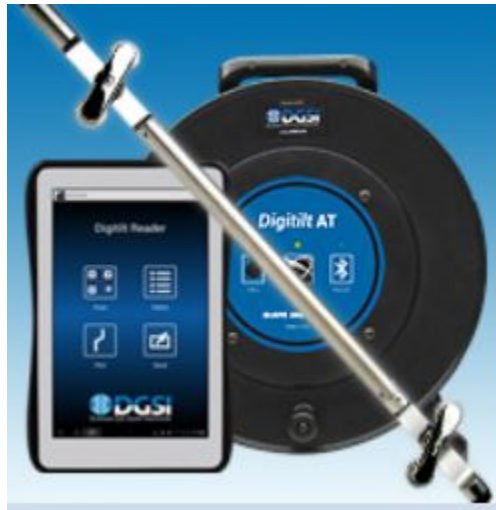
Figure 9-2 Digitilt AT slope inclinometer system [5]
