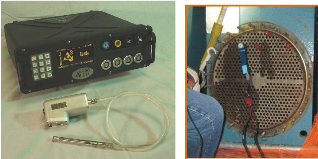
Figure 5-2 Two Ultrasonic Guided Wave Probes for Tube Inspection
