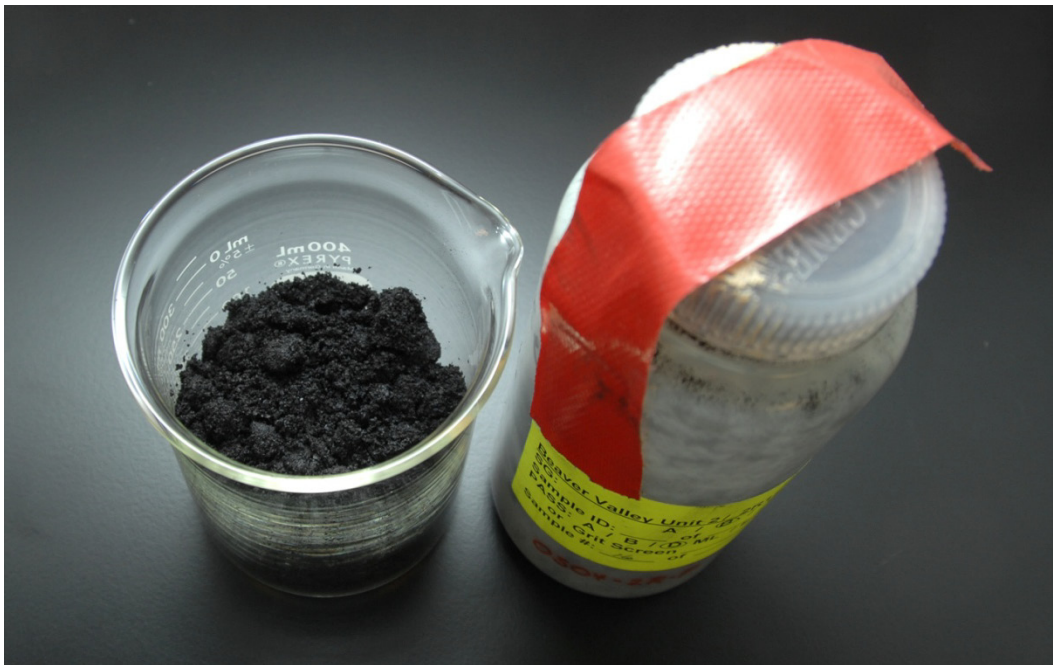
Figure 2-2 Typical Nature of As-Collected SG Deposit Samples
