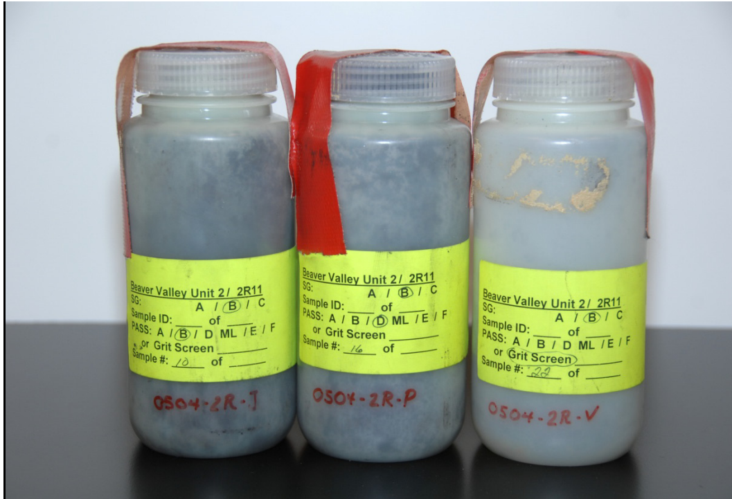
Figure 2-1 As-Collected SG Deposit Samples
