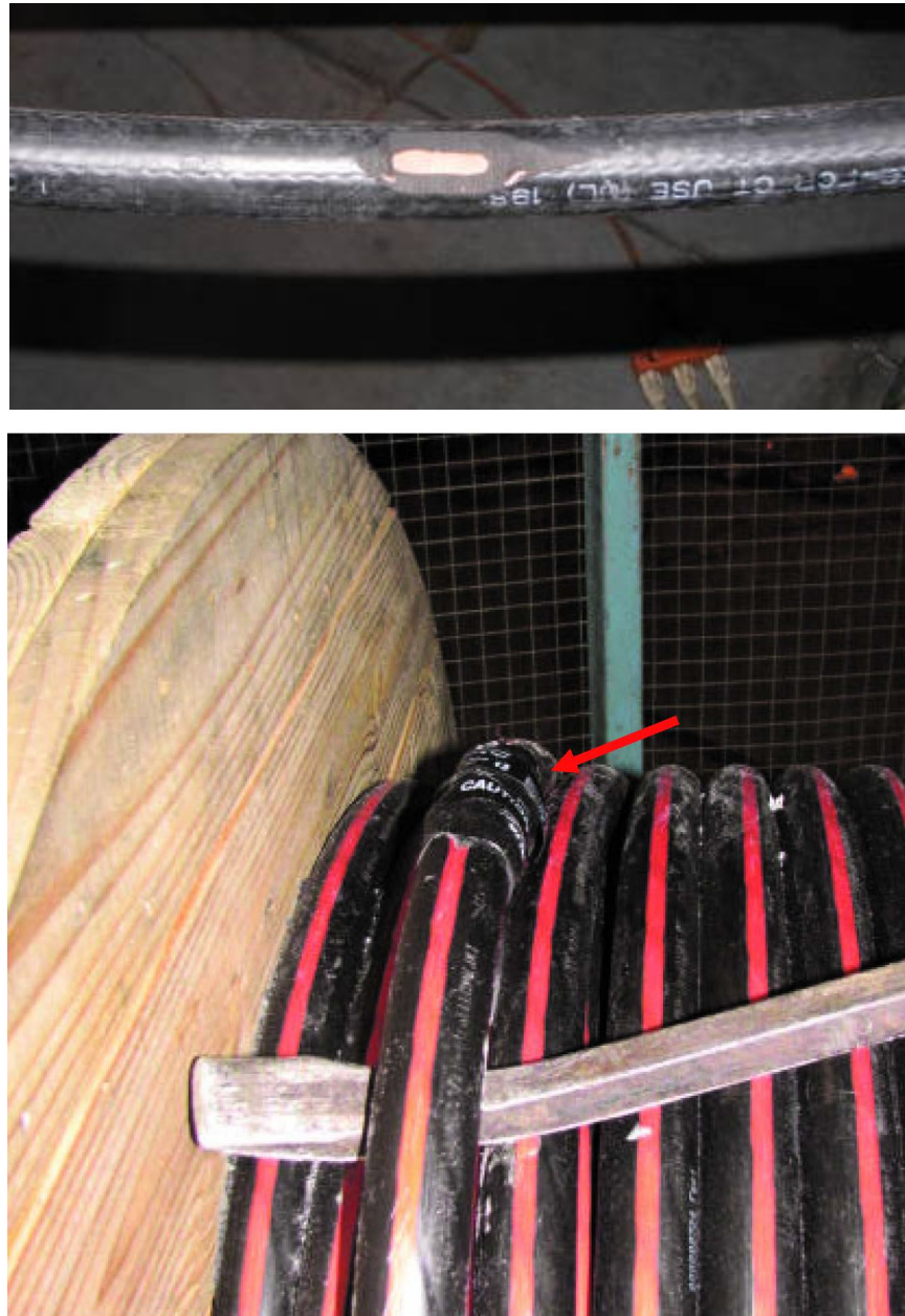
Figure 2-4 Artificial cable defects, introduced to serve as the source of partial discharges
