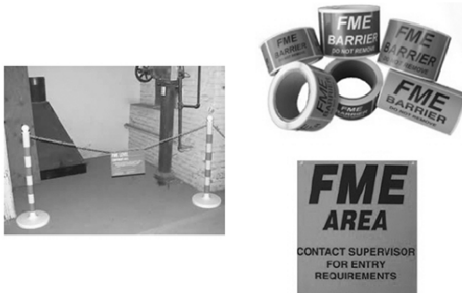
Figure 3-1 FME signs and barriers
