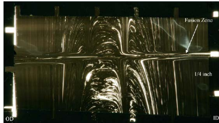
Figure 4-12 Photograph of a 25 – 35 micron slice from the fusion zone of unevenly mixed PE3408 HDPE pipe
