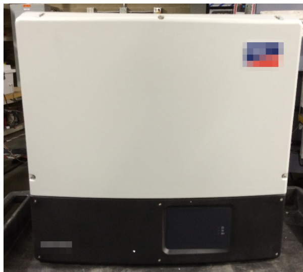
Figure 1-1 Three-phase Inverter used for LRO and GFO Testing
