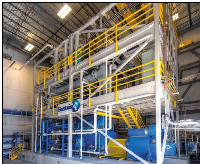
Figure 2: SustainX's 1.5-MW 40-minute prototype (Source: SustainX)
