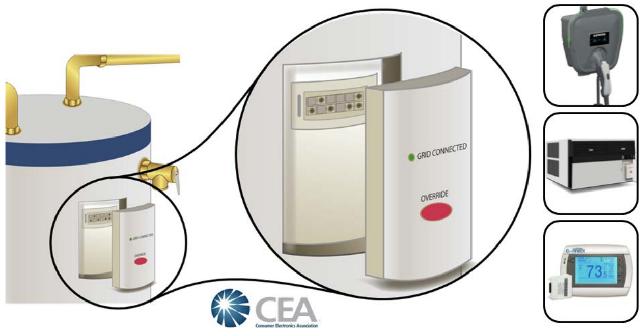
Figure 1-1 Concept of the CEA-2045 modular communication interface
